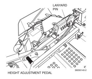
Figure 4-5. Adjusting Cutting Height
